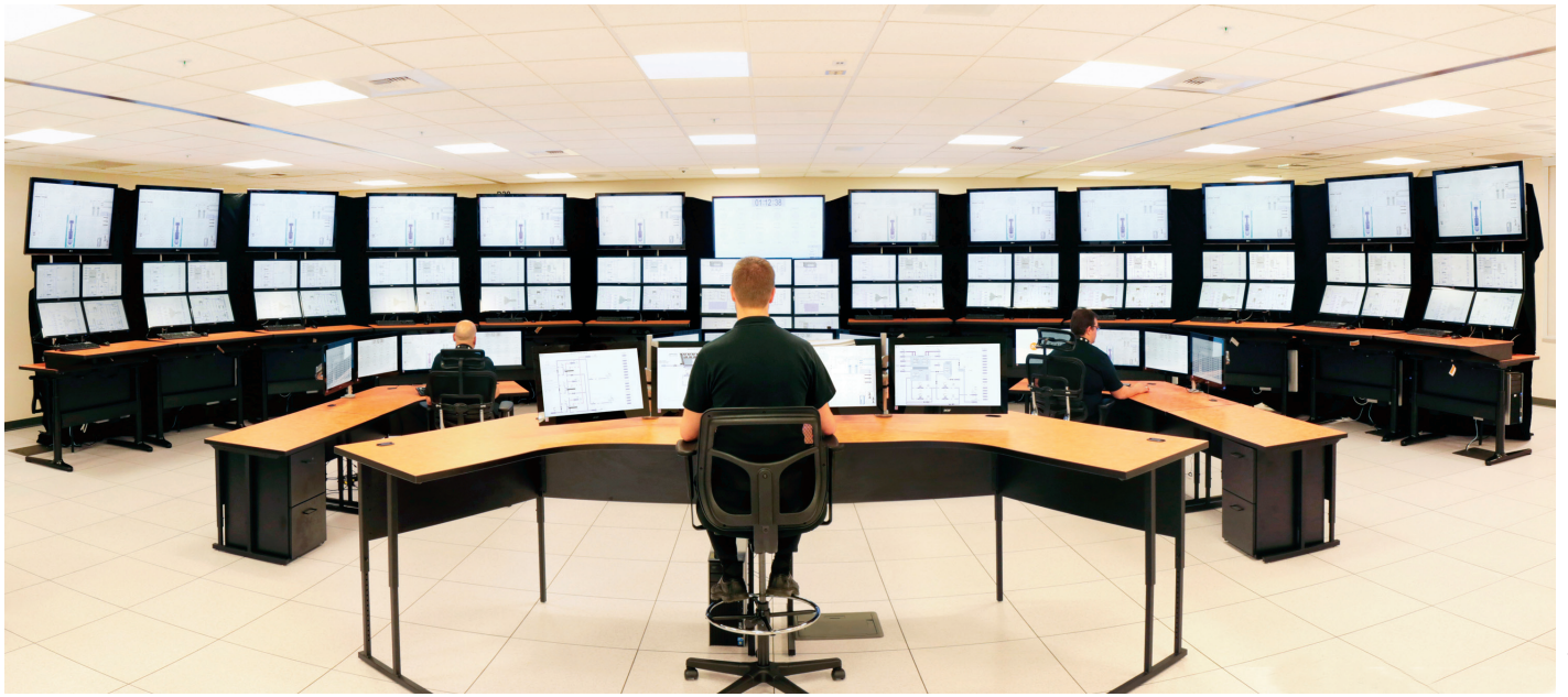
The NuScale Power Control Room Simulator is designed to simulate the operation of a 12-module NuScale power plant.
