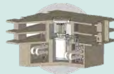
KP-FHR Fluoride salt-cooled high-temperature reactor KAIROS POWER
