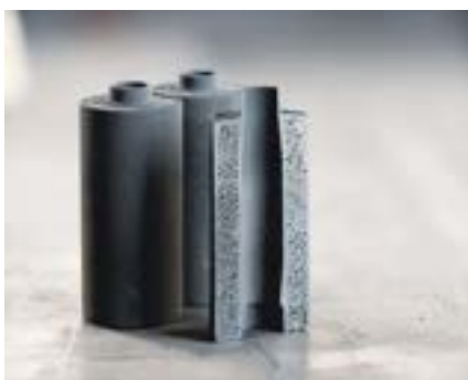
Figure 1: Example of TRISO fuel developed by advanced nuclear reactor companies USNC and X-energy
