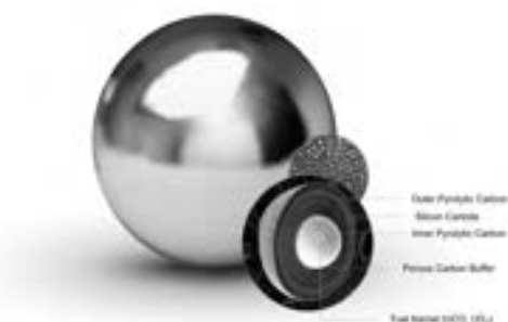
Figure 1: Example of TRISO fuel developed by advanced nuclear reactor companies USNC and X-energy
